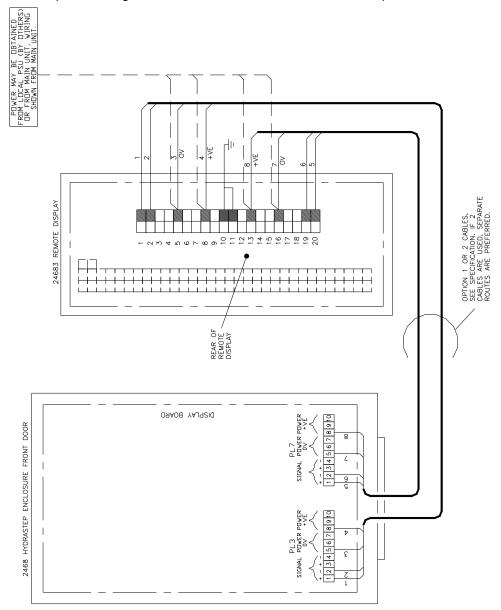
Figure 4.2 - Interconnection cable for a single remote display
